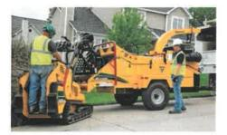
ENGINE OPTIONS. The BC1500 is offered in either a 165 hp (123 kW) PSI 5.6L gasoline engine and 130 hp (97 kW) Cummins QSF 3.8L Tier 4 Final engine.
